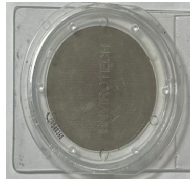
Fig 3.7 PM 2.5 filter paper after sampling
