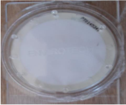
Fig.3.6 PM 2.5 filter paper before sampling
