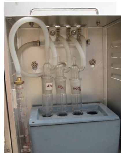
Fig.3.5. Impinger tubes connected with Air flow meter
